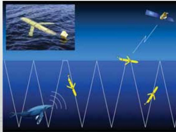
An autonomous glider moves up and down in the water column in a sawtooth pattern while detecting, recording, and identifying marine mammal sounds. Upon surfacing, the glider transmits detection and identification data to shore via satellite.
