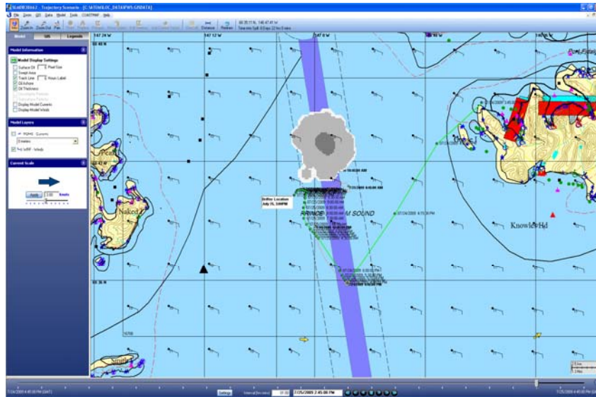
Fig. 51. ATOM comparison of oil spill trajectory forecast at 3:00 pm (Grey regions) July 25 with drifter location (white label). Oil Spill Forecast created with ROMS currents.
