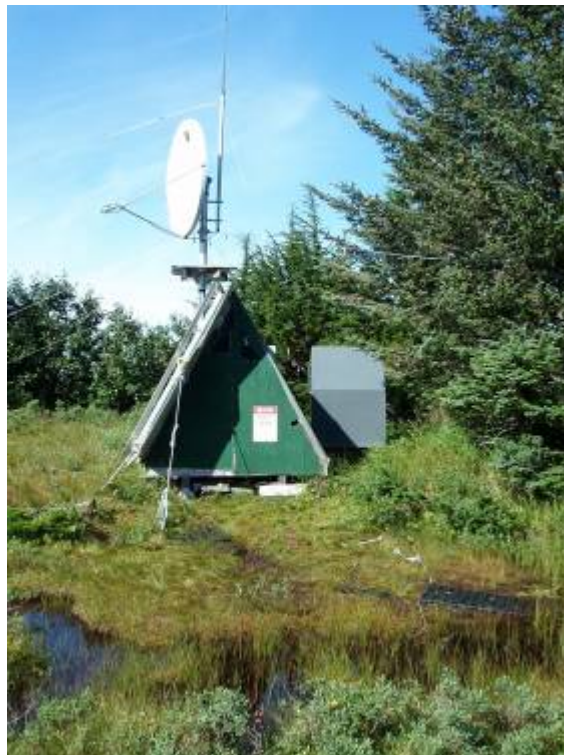
Fig. 13. HF radar as deployed in Prince William Sound.
